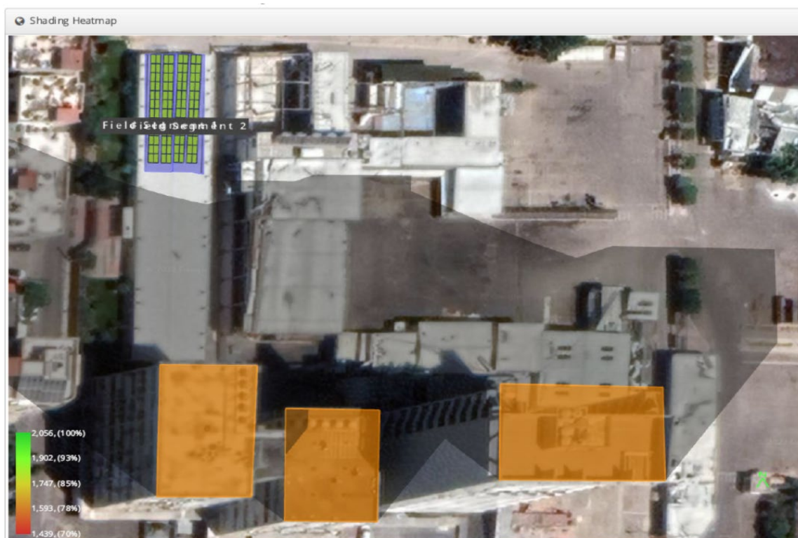
Figure 4 – Shading Simulation for solar PV Panels
